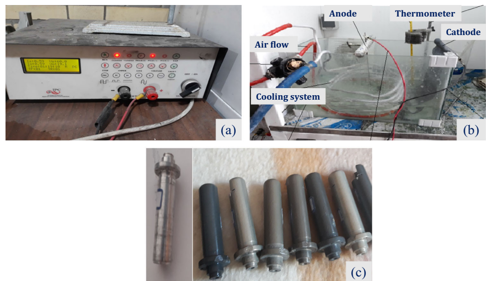
Fig. 1 Anodizing setup a power supply, b cooling system and c aluminum sample pre- and post-anodizing
