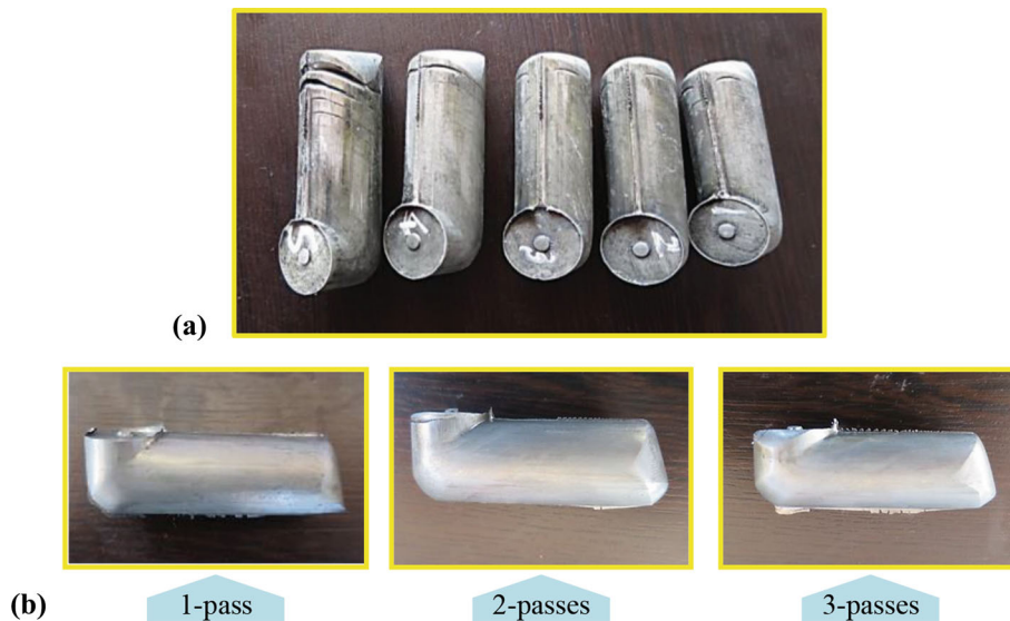
Fig. 3 ECAP-treated samples after (a) solution treatment and appeared cracks for one-pass and (b) Annealing treatment for 1, 2, and 3 passes without any cracks
