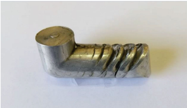
Fig. 2 Cracked sample after performing the ECAP process at room temperature
