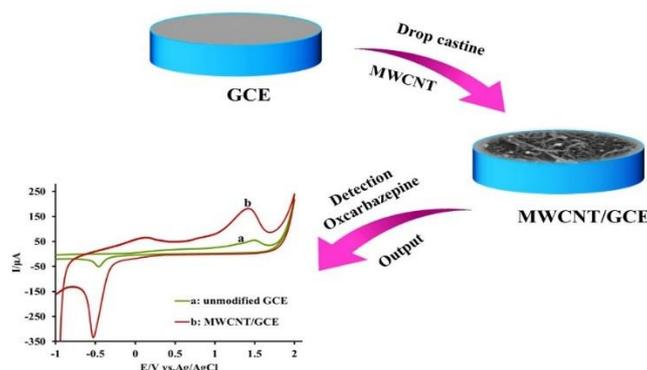
**Figure 2.** Schematic of modified electrode preparation
