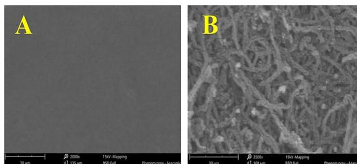
**Figure 10.** (A) Scanning electron image of unmodified glassy carbon electrode; (B) Electrode surface covered with carbon nanotubes
