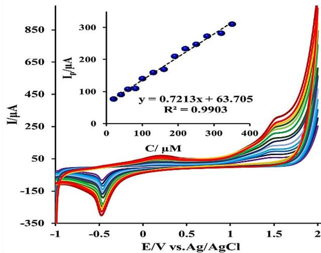
**Figure 6.** Plot of concentration versus current for oxcarbazepine
