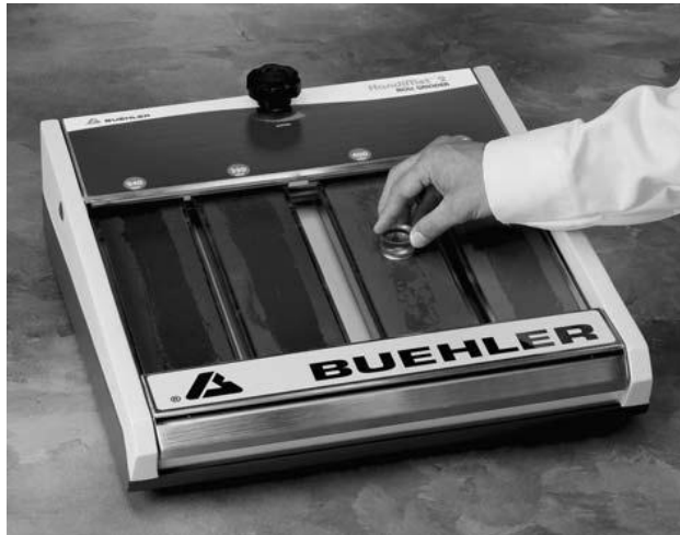
Hand grinding using a simple hand grinding device.
