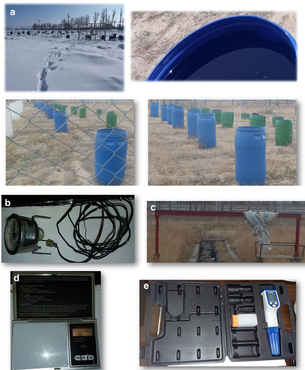
Fig. 1 Study area, (a) barrels, (b) thermometer, (c) weighbridge ) to measure the salt weight of the barrels), (d) scale (to measure the water sample), (e) electrical conductivity (EC), total dissolved solids (TDS) meter (f) on the left-hand side; rain gauge and on
