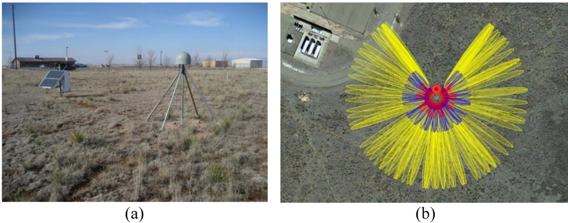
Figure 12: (a) Photograph of a GPS site, called P038, in Portales, New Mexico. The antenna phase center at this site is approximately 2 m above the soil surface. The station has been installed since 2015. (b) Google Earth image for PBO site p038 and reflection zones for 2-m RH and satellites with elevation angles between 5° and 15°.
